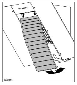
First fit the top of the grease filter into the slots at the top, then swing the bottom of the grease filter into place and press it into position.
