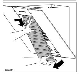
Pull the grease filter carefully out of its mountings along the bottom edge. Then pull it towards you a little whilst pressing it in at the top. It can then be taken downwards to remove it.
