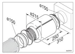
To achieve even further reductions in noise levels, a special silencer (optional accessory) can be fitted in the ducting system.
