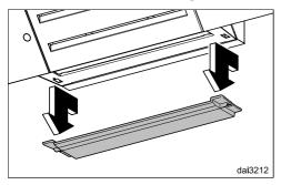
Pull the drip tray forwards a little, and then pull it downwards to remove it.
