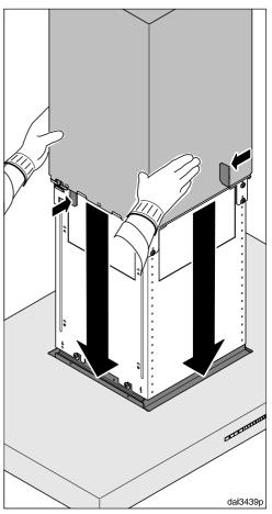
■ Hold the tower securely, bend back the retaining tabs and carefully lower the tower.
