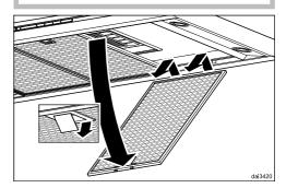
■ To take out a grease filter, release the locking clip on the filter, lower the filter approx. 45°, unhook it at the back and remove it.
