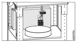
■ Connect the mains cable. See "Electrical connection".
