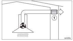
In extraction mode, the silencer not only reduces noise from the fan outside the house, but also sounds originating outside reaching the kitchen through the exhaust ducting (e.g. traffic noise). For this reason, the silencer must be positioned as close as possible to the ducting exit ①.
