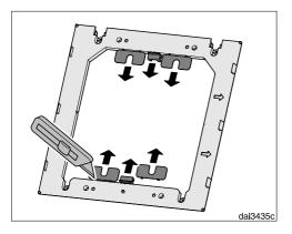
Use a knife to release the four spacers and the two covers from the spacer frame supplied.
