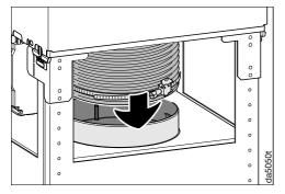
■ Slide the vent ducting onto the vent socket and secure it (using a hose clip, for example).
