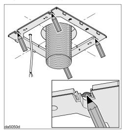
■ Use the spacer frame as a drilling template. Place it on the ceiling with the arrows pointing forwards. Using the notches, align the spacer frame on the intersecting lines and make pencil marks for the drill holes.
