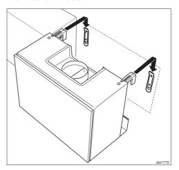
■ Hang the cooker hood into position using the adjustable brackets.
