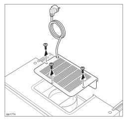
■ Remove the recirculation grille for extraction mode.
