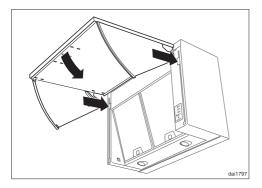
Attach the vapour canopy with cabinet door fitted and then close it.
