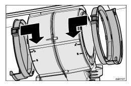
■ Fitting for the first time: fit an adapter onto each side of the fan and turn to secure position in their holders.
