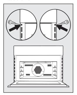
■ Open the door with the sensor control and use the screws supplied to secure the oven to the side walls of the housing unit.
