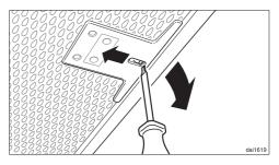
If a grease filter is inadvertently replaced upside down, insert a small screwdriver blade into the slit to disengage the clip.
