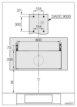
When installing a custom back wall with pre-drilled holes, please refer to the drilling distances in the drawing above (screws Ø 5 mm).
