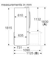
A: Front is adjustable from 1830 to 1847, with front levelling feet fully extended **B**: With handle
