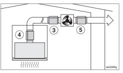
For operation with an external motor, noise from the motor outside the house and inside the kitchen can be minimised.
