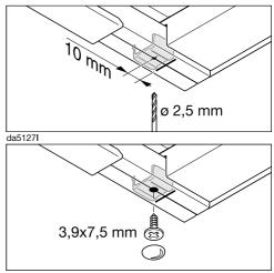
Drill a pilot hole 10 mm in front of the pen mark and screw the depth stop into place.
