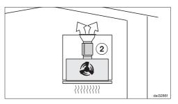
In recirculation mode, the silencer needs to be positioned between the exhaust vent and the exhaust grille ②. Check that there is sufficient space.
