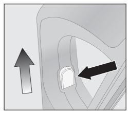
Press the release catch and remove the Comfort handle by pulling it upwards.
