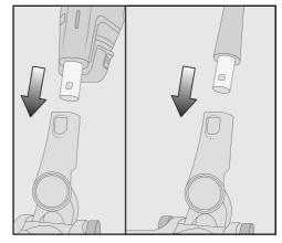
Push the connector into the Electrobrush from above until it audibly clicks into place.
