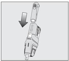
The PowerUnit can be used on its own (PowerUnit solo) without the suction tube and Electrobrush as a quick way of vacuuming up crumbs and fluff in specific areas.
